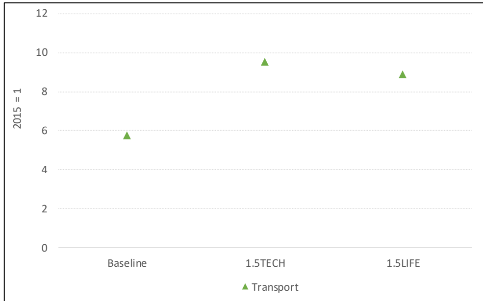
Figure 2-5. Ratio between 2050 and 2015 electricity consumption in transport in the Baseline, 1.5TECH and 1.5LIFE scenarios Source: PRIMES model, E3-Modelling
